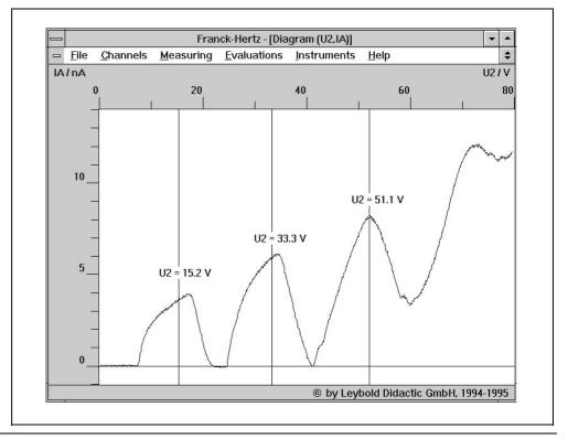
Fig. 4: Franck-Hertz curve for neon (recorded using an XY-recorder)
